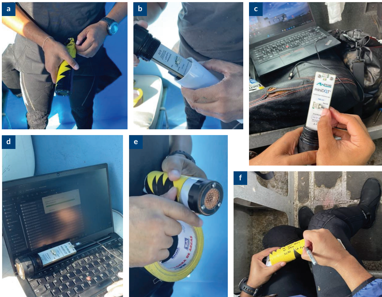
Figure 2. Sensor maintenance and data upload procedure once the sensor has been retrieved: (a) the sensor retrieved, (b) taken out of its protective case, (c) connected to a computer for (d) downloading data, (e) placed back in the case and covered in bright tape, and (f) dated.
