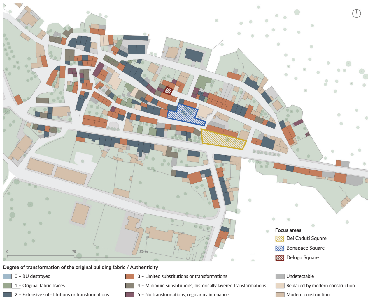
Figure 2. Visual map of the degree of transformation of the original building fabric.
