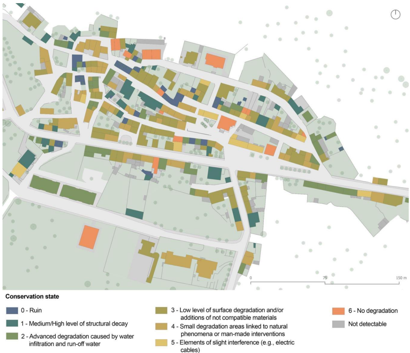
Figure 1S. Visual map of the conservation state of the BUs. The parameter goes from the maximum degradation of the building (0 - building in ruin), to no degradation detected (6). The map was built using data from direct observation of the built fabric and the photographic campaign. Source: authors.
