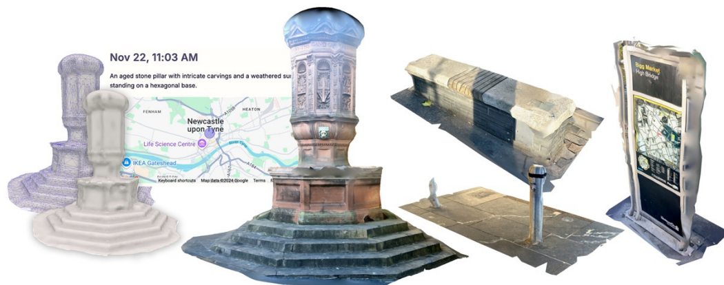
Figure 10. Extract from LiDAR scanning of temporal objects in the study area using a hand-held device and using the professional Polycam LiDAR scanning platform for analysis and digital sharing, with an extract of timestamp/geolocation metadata.
