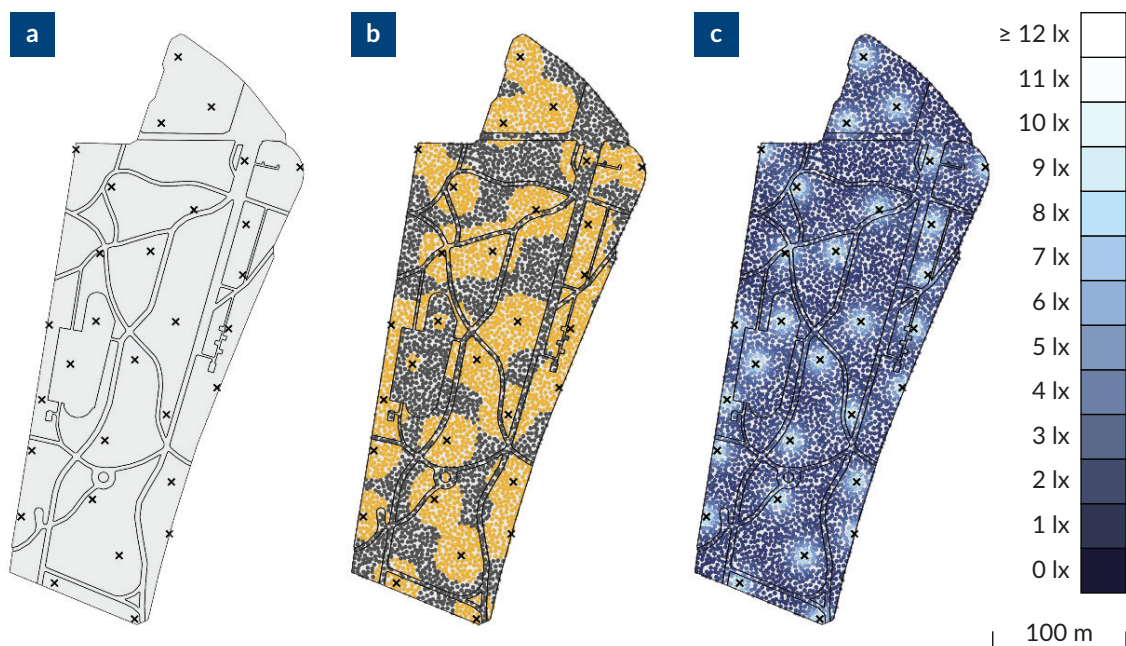
Figure 4. The initial state of simulation: a) initial positions of lamps, b) visualization of test points meeting the minimum illuminance criteria (orange samples) and being under-illuminated (dark grey samples), c) visualization of test points computed illuminance levels.
