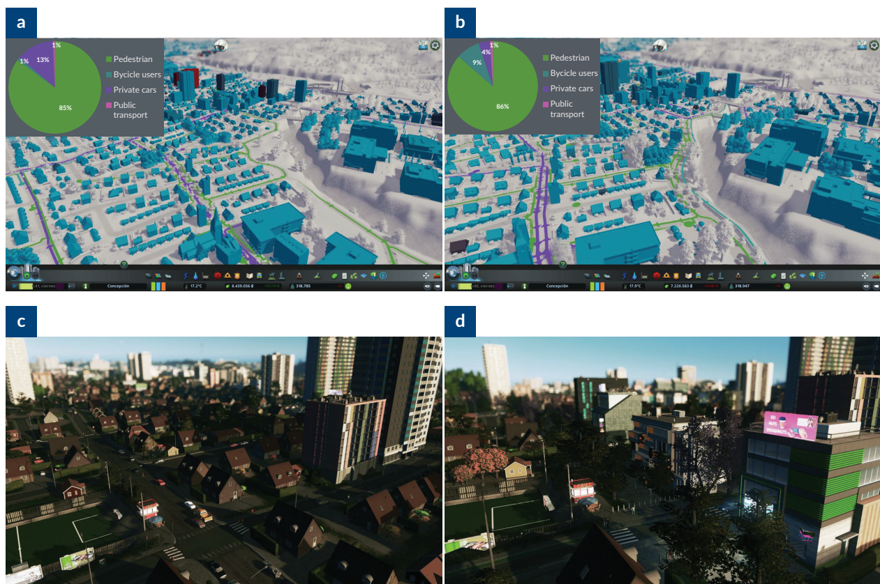
Figure 8. Comparison of game-based simulated scenarios in C:S: (a) base routes and modal split; (b) resulting routes and modal split after simulated variations; (c) geospatial view of the base scenario; (d) geospatial view of the modified scenario with an updated built environment.
